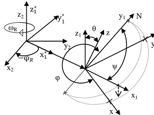
Fig. 3. Adequate systems for the motion of a steady point on the ball surface.
