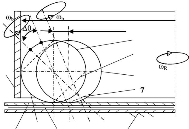
Fig. 2. Nutation of the ball own rotation axis.
